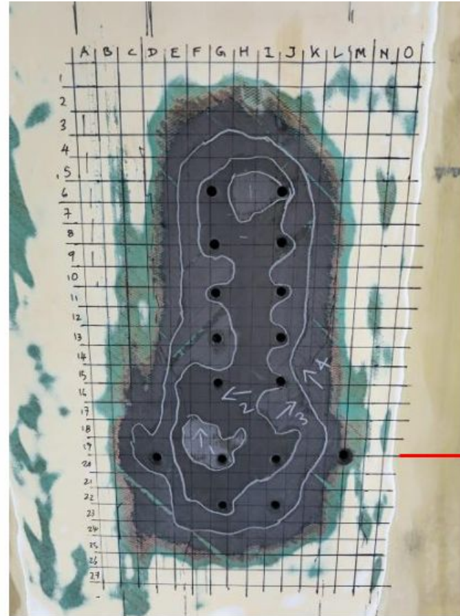
Grid Mapping with over 400 measurement points
