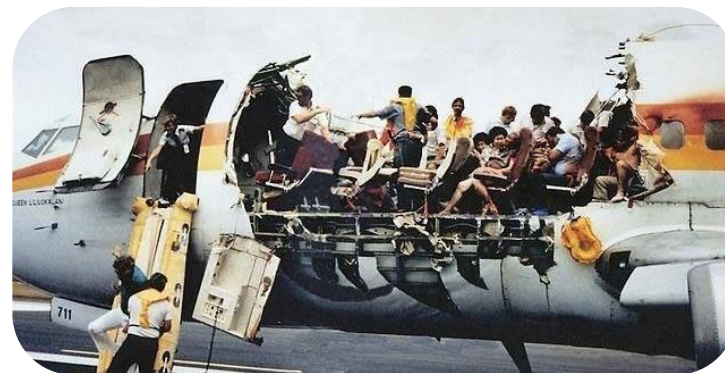
Aloha Airlines Flight 243 - Boeing 737-200 - 04/1988 Cause: fatigue cracks + corrosion [2]
