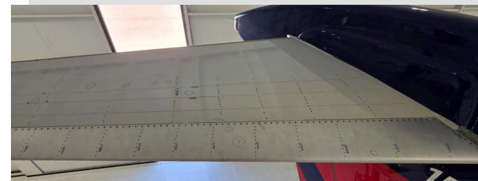
Damage location overview on RH H-stab upper skin, RHS
