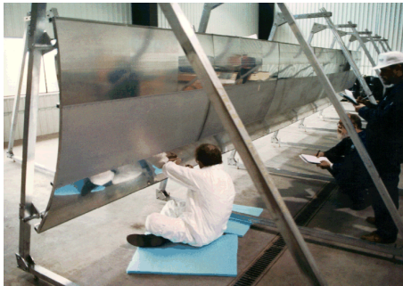
Small Crack/WFD Panels
