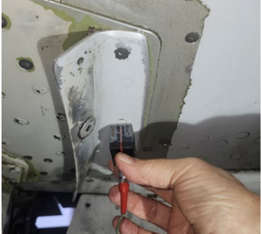
PROBE NULL/BALANCED ON FAIRING ATTACH ANGLE AND EDM NOTCH INDICATION TYPICAL FOR FASTENER HOLE NO's: 1, 3, AND 6
