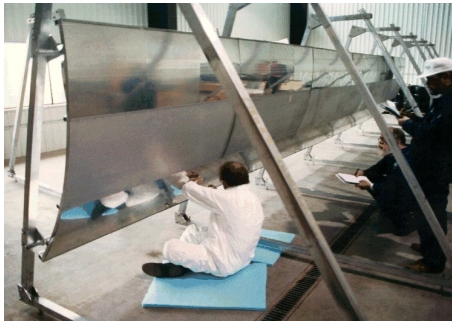
Small Crack/WFD Panels
