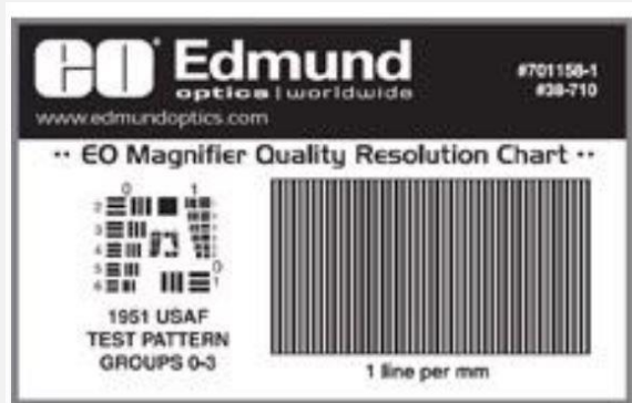
USAF-1951 Resolution Target
