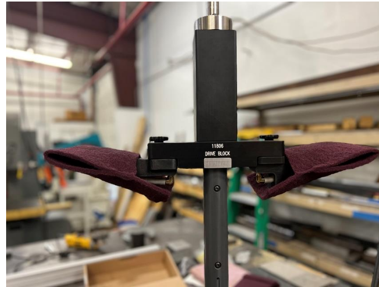
Compliant Paddle Design for Cones
