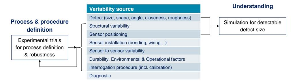
Process & procedure definition: experimental trials to define the inspection procedure, including calibration and detection criteria
