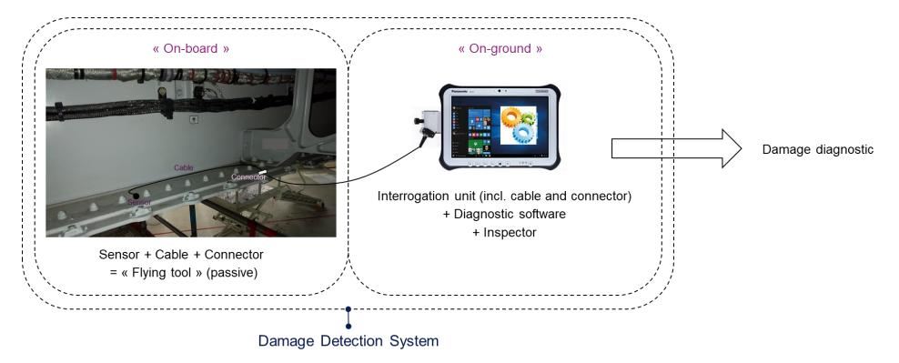
The damage detection system is composed of the full chain of inspection (sensor, acquisition and diagnostic)
