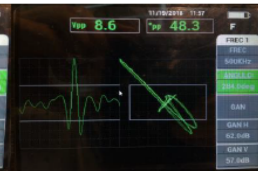
Steel with crack
