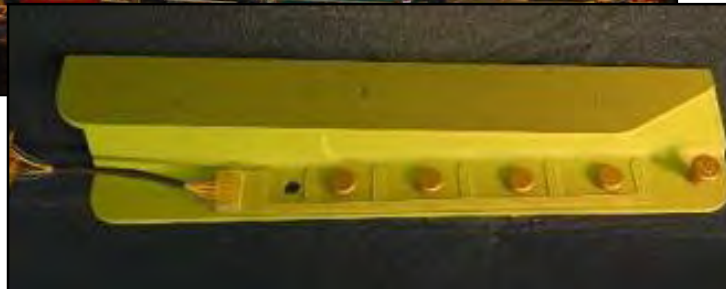
CVM Sensor Installed on Structure to be Monitored
