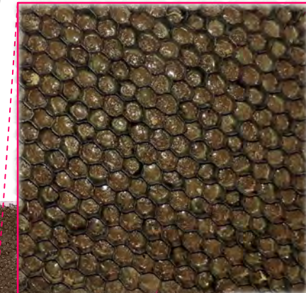
Repair 9b Core Sectioned Top Skin
