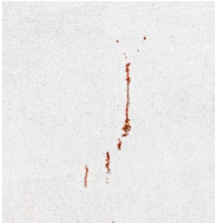
Picture of penetrant indications
