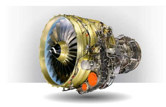
CFM SB's 72-0568 and 72-0579 provide the inspection details for the repetitive on-wing eddy current inspections. SB effectivity is dependent upon TRF part number. AD is applicable only to part numbers in SB 72-0579.
