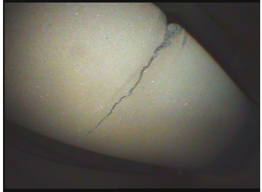
CFM56 LPT Vane Segment Older Borescope Resolution
